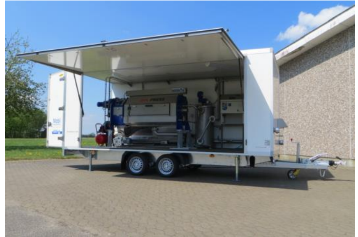
Assens Forsyning, Denmark - Mobile sludge dewatering unit with SP-HF04 screw press
