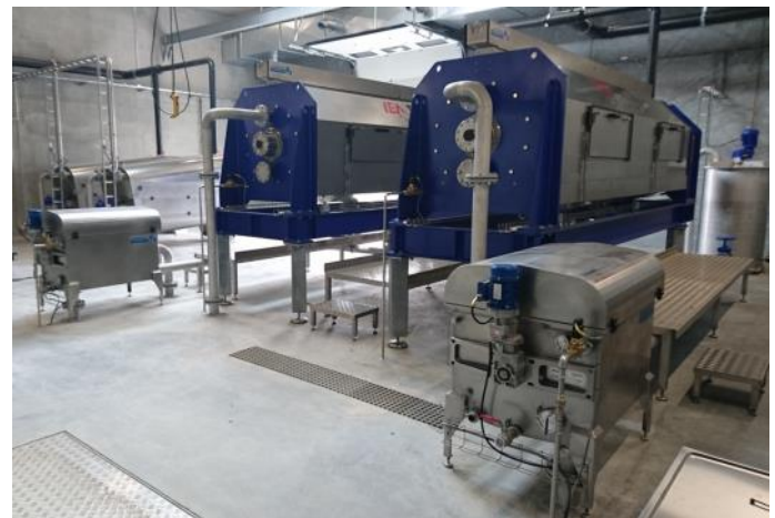
Solrødgaard, Hillerød, Denmark - 2 pcs SP-HF08XL screw press and MF600 Microscreen filtrate filtering
